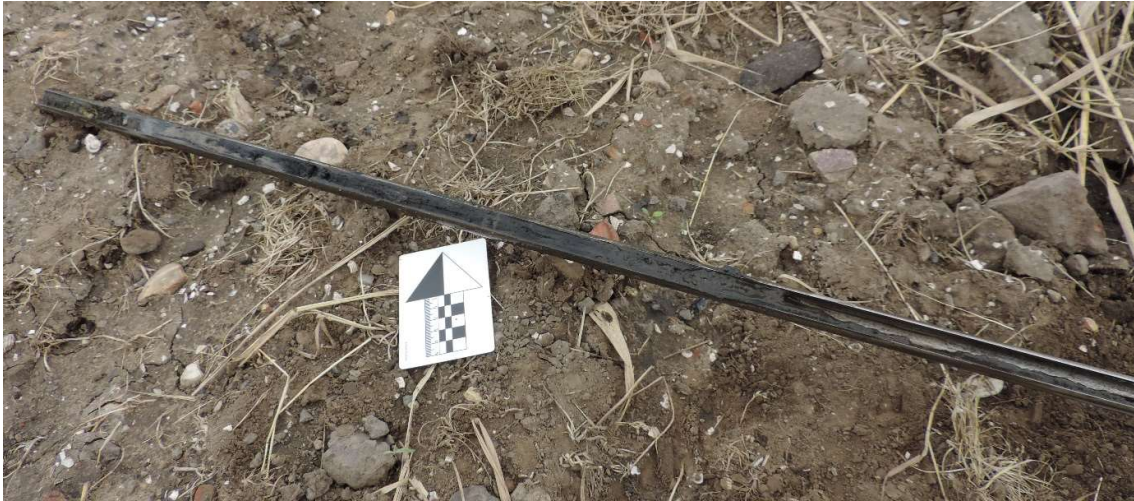
Figure 42 - Auger sample – sequence Auger 09 (image number: DSCN0722) In this sample, there was blue-grey clay to 1.3m, followed by organic matter
